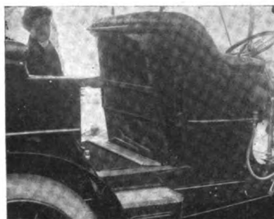
FIG. 4.—SPECIAL SEATS OF LOCOMOBILE STOWED UNDER FRONT SEAT.
